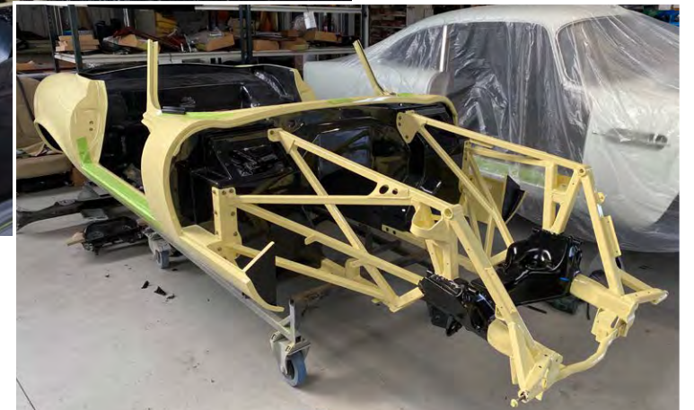
Below. The completed chassis, with the carbon tub and steel frame
