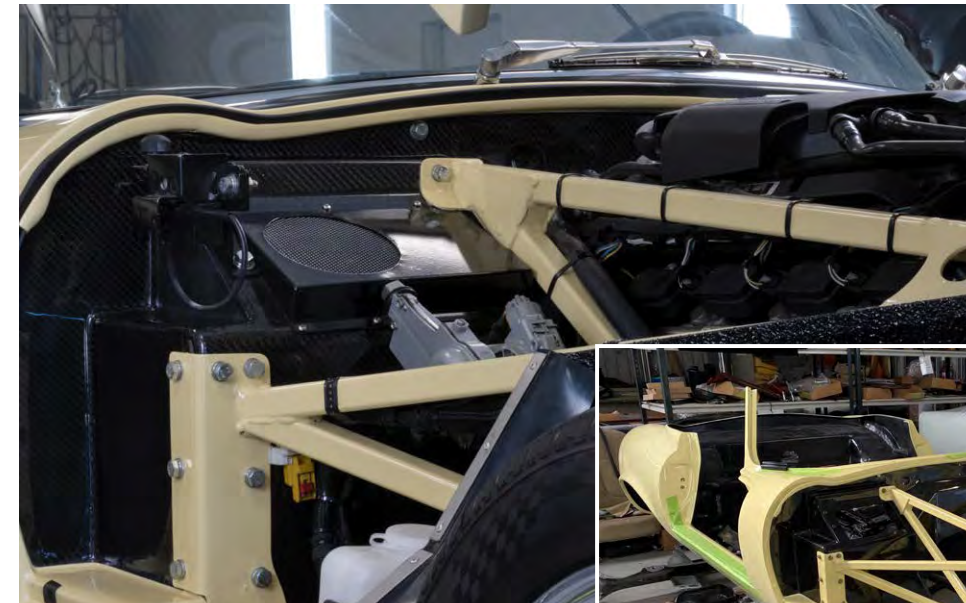
Left. Integration of the steel front end to the carbon fire wall
