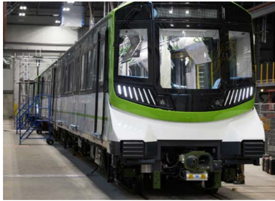
For Alstom India - REM Driver cab and carriage with GRP front end, interiors and exteriors.
