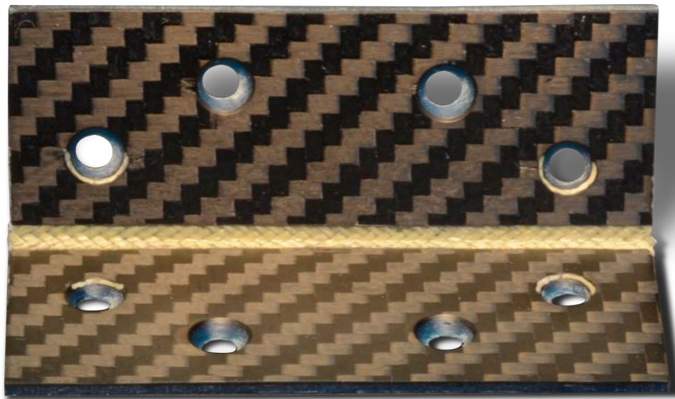
Co-moulded carbon-kevlar hinge integrating rigid composite wings with a flexible centre section, eliminating the need for mechanical fasteners.
