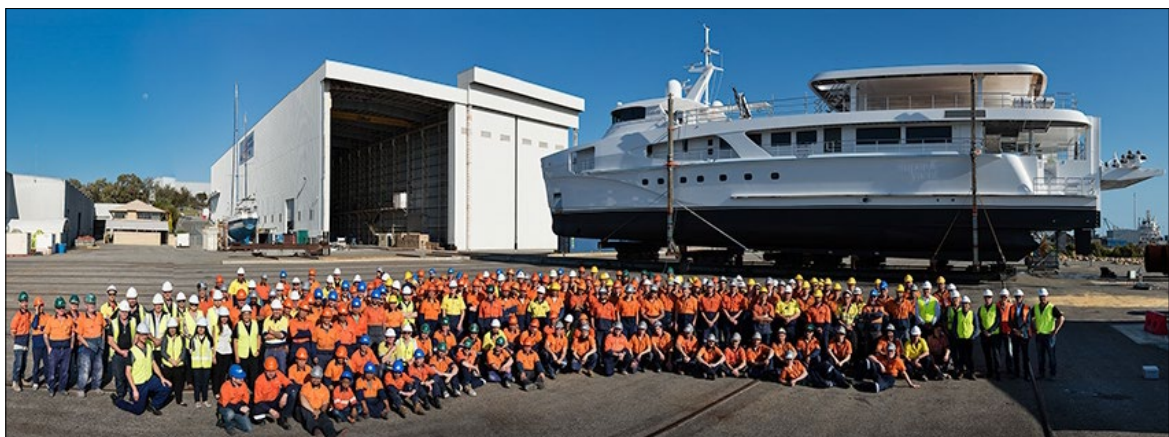
Launched in 2016, the 46-metre composite twin-hulled yacht 'Charley' remains one of the largest composite, resin-infused multi-hulls in the world. The 3D design and construction of the bespoke vessel took two and a half years (by Echo Yachts). Notably, these projects are important for employment and skills.
