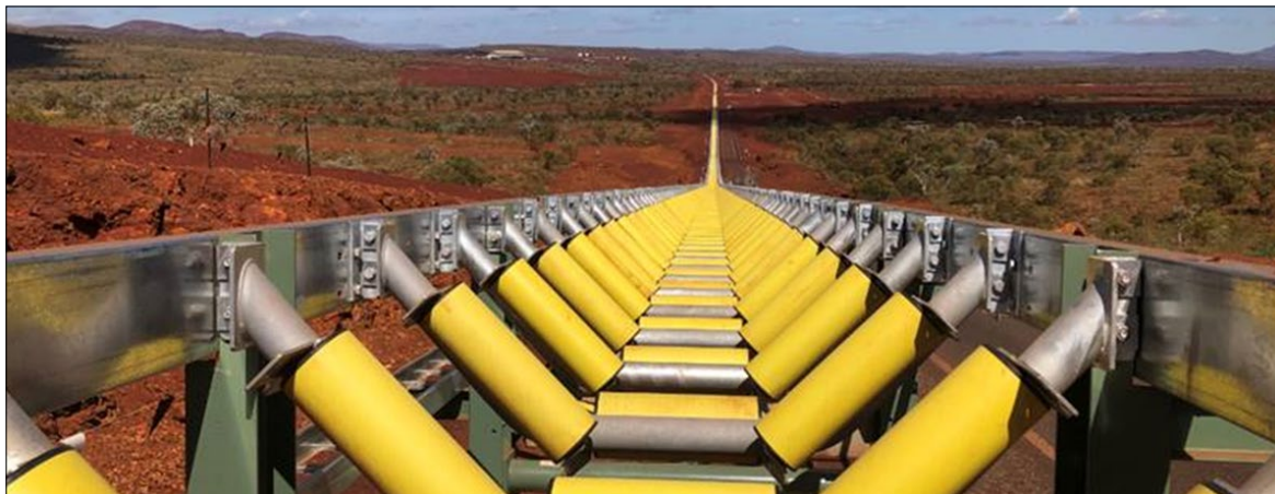
CPS supplies BHP South Flank overland conveyors with Pilbara's first all-composite roller solution.
