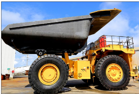
Prototype of a carbon fibre tray for 150 tonne Haulpak dump truck fitted with an MRL carbon fibre tray. The West Australian reported on April 14 ‘MinRes puts CarbonArt on ice amid coronavirus pandemic’
