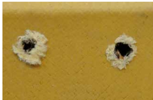
Drilling Operation Damage of Kevlar Structure (photo by Rik Heslehurst)
