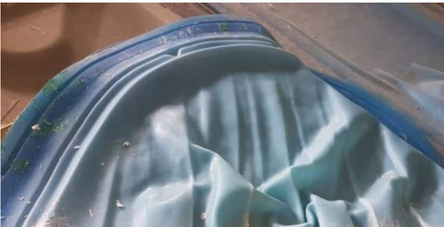
Figure 5: Illustration of ACC Silicone membrane condition after 1200 plus uses with polyester resin moulding
