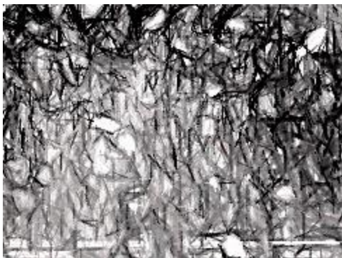
Figure 7 – Above is an electron microscopic image of a worn-out silicone surface through styrene attack.
