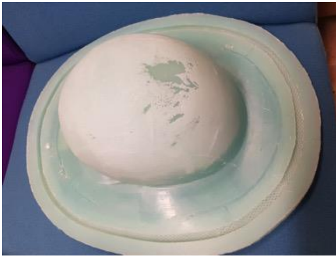
Figure 6: A different European silicone supplied illustration of a riding helmet membrane after only 160 cycles using polyester resin. Note the surface peeling where the part has stuck and rendered the membrane unserviceable after such a short production run
