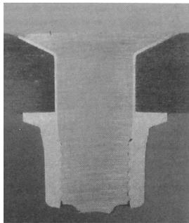
Countersunk fasteners will typically reduce the bearing strength due to a relative increase in the fastener tipping. The fastener tipping can also initially cause delaminations if not sized and drilled correctly. Such issues are of major importance with thin structures. The introduction of a knife or feathered edge will result in delaminations in a short period of time.
