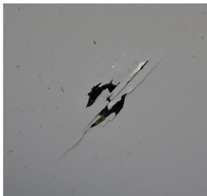
Hole Back Surface Delamination Damage from Drilling
