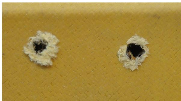
Drilling Operation Damage of Kevlar Structure
