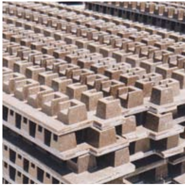
Capping boards for electro-winning cells installed at MICC Copper Refinery, Burma
